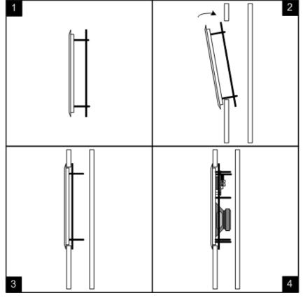
cut-out. The white frame should fit snugly and smoothly in the cut-out hole. If the hole should have been cut a little too large, the flange on the frame should cover this.
